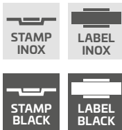
Double-sided embossing width 25 mm with inlay in INOX finish or painted black. The inlay may be placed either on one or on both sides. It is placed in embossing and flush with the leaf (STAMP) or boned to a flat leaf (LABEL).
