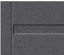
Double-sided embossing width 25 mm, depth 2 mm.
